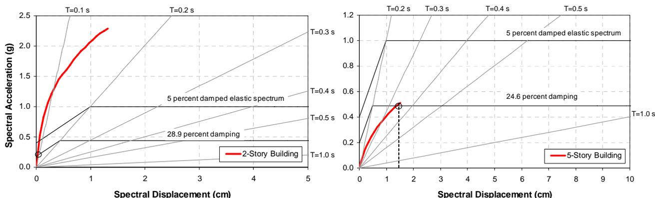
Figure 5. Capacity spectrum method to the 2 and 5 story buildings based on the Turkish Seismic Code (1998) design spectrum (soft soil site condition)
