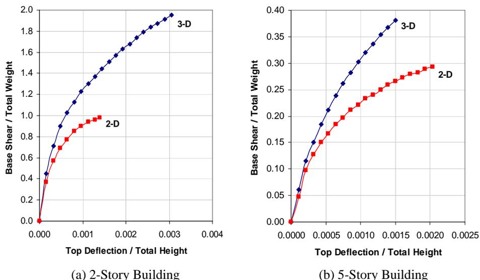
Figure 4. Modified capacity curves for 3D and 2D models
