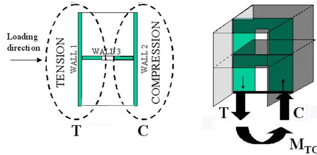
Figure 6. Slap-wall interaction due to tension and compression (T/C) coupling mechanism
