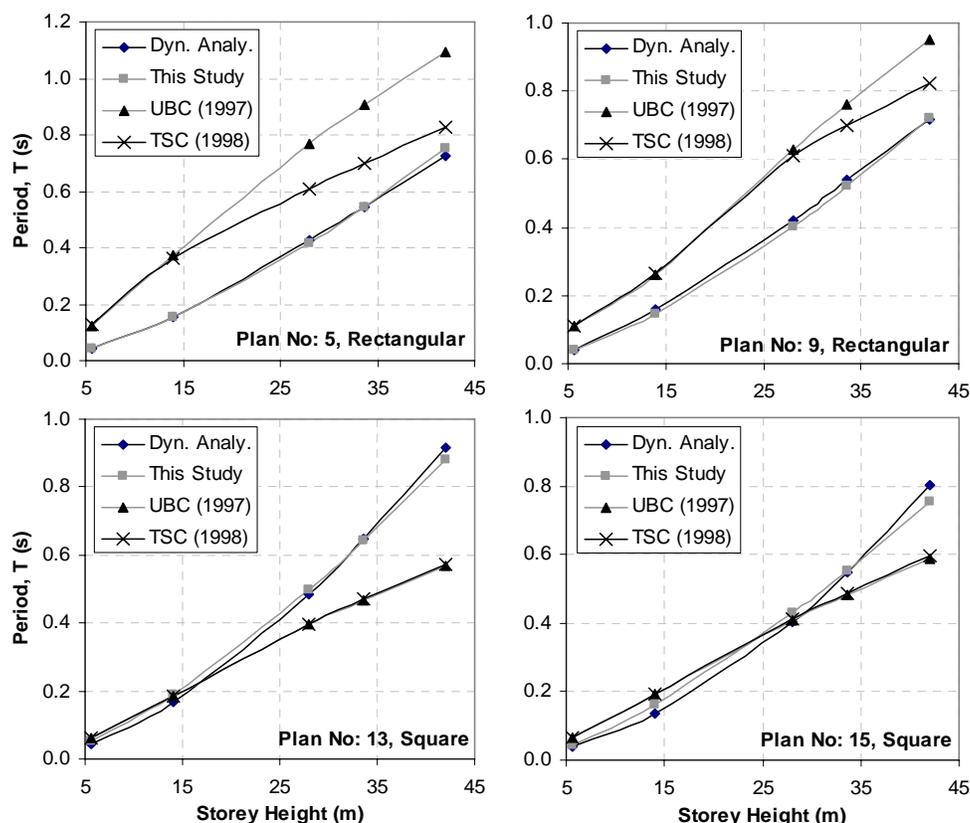
Figure 2. Comparison of fundamental periods for various heights of rectangular and square plans
