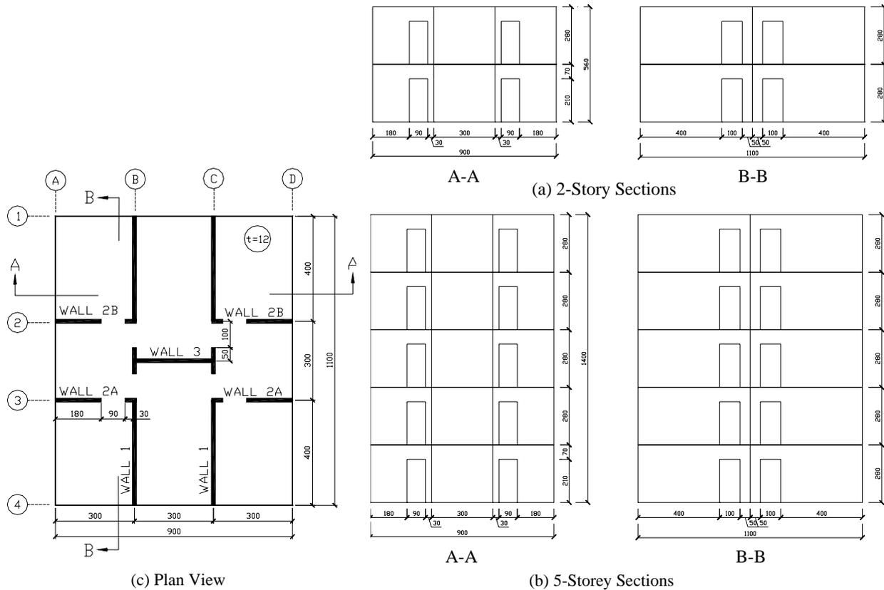
Figure 3. Typical architectural plan and section views of the 2 and 5-story buildings (units are in cm)
