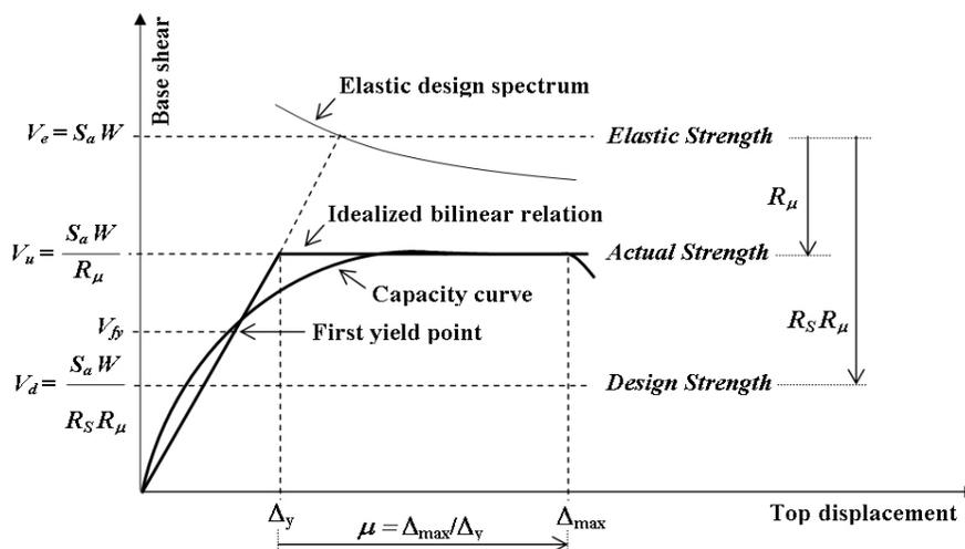
Figure 9. Relationships between the response modification factor ( $R$ ), ductility factor ( $R_{\mu}$ ) and overstrength factor ( $R_S$ )
