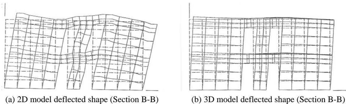
Figure 7. Deflected shapes for *Wall 1* in 2D and 3D models for 2-story building
