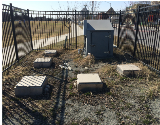
Free-field surface station and downhole array with six boreholes
