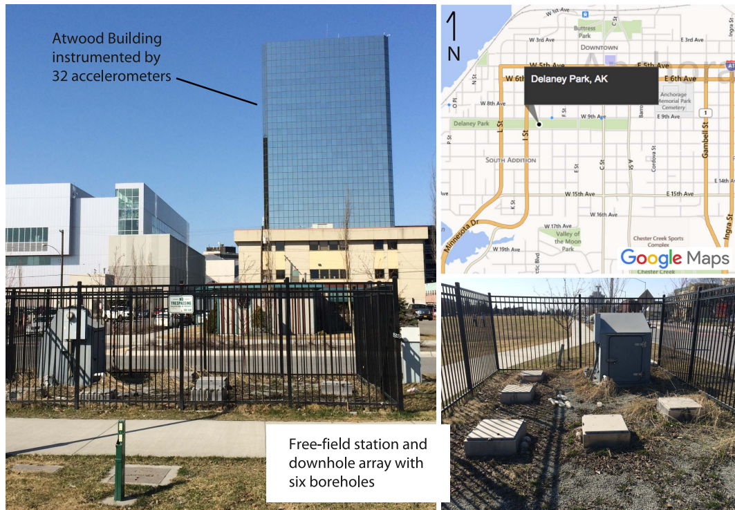
Fig. 1. DPK borehole array in downtown Anchorage, Alaska. The Atwood Building (20-story steel moment frame) in the background (165 m away from DPK array) is also instrumented. The map insert shows the location of Delaney Park. (Map data © 2020 Google, images by Erol Kalkan.)
