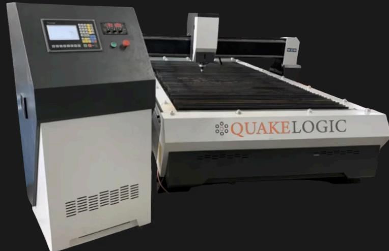
The **QL-Plasma Pro** is an industrial-grade **CNC plasma cutting system** designed for high-precision cutting of carbon steel, stainless steel, aluminum, and other conductive materials. Built on a **rigid welded steel structure**, it combines advanced motion control, intelligent height tracking, and seamless CAD/CAM workflow for dependable production in manufacturing, research, and educational environments.
