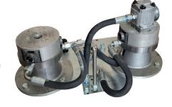
On the dual stage pump, a high delivery, low pressure gear pump is used for rapid approach, for quick gripping the rebar while a low delivery, high pressure radial piston pump is used for 400 bar grip pressure.
