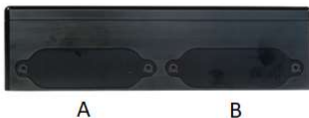
Figure 2 – Position of the Atlas batteries. A) primary battery slot, B) secondary battery slot
