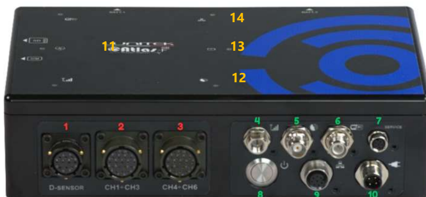
Figure 7 – Atlas Plus connections and lights
