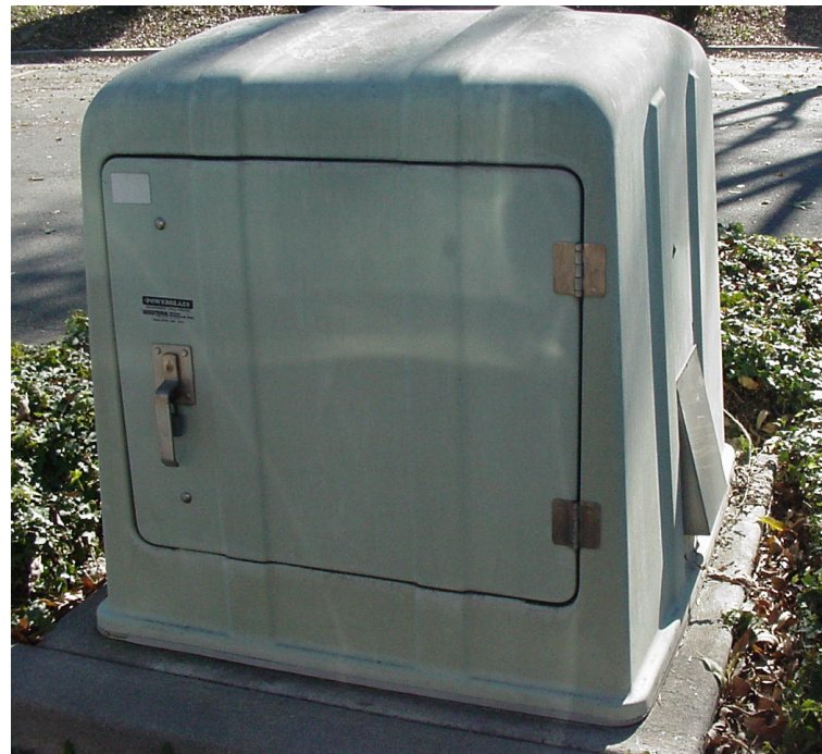
Figure 1. Photograph of a typical free-field station where a triaxial accelerometer and a recorder are installed to measure ground motion away from structures that are being seismically monitored (U.S. Geological Survey photograph).
