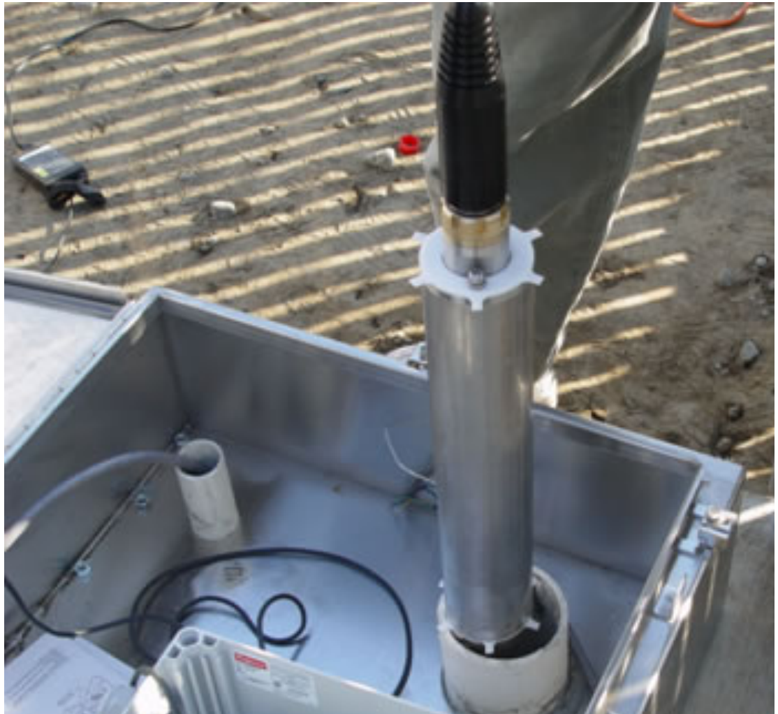
Figure 4. Installation of downhole sensor into the tubing (USGS photo)
