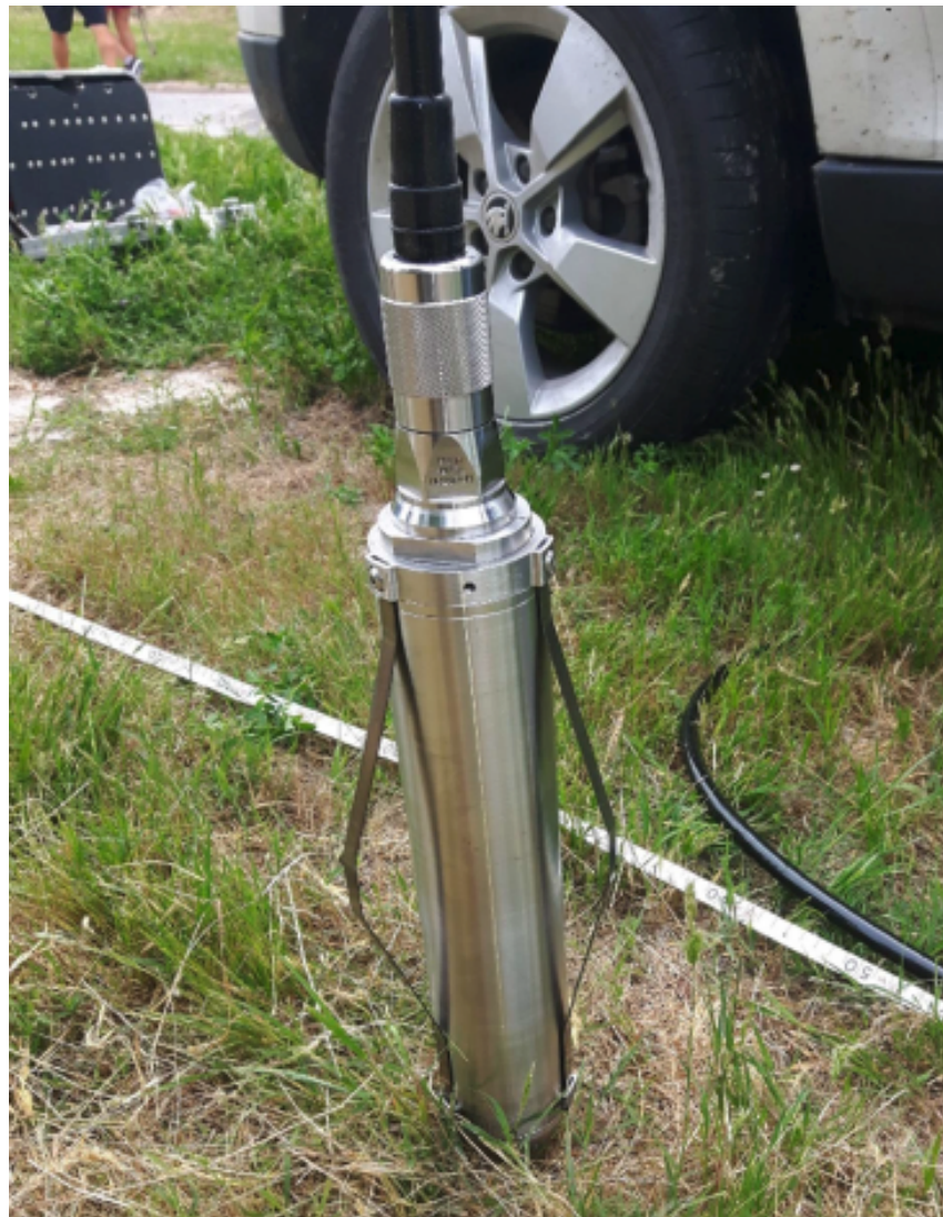
Figure 1. An example borehole accelerometer —TELLUS BOREHOLE (Lunitek Photo)
