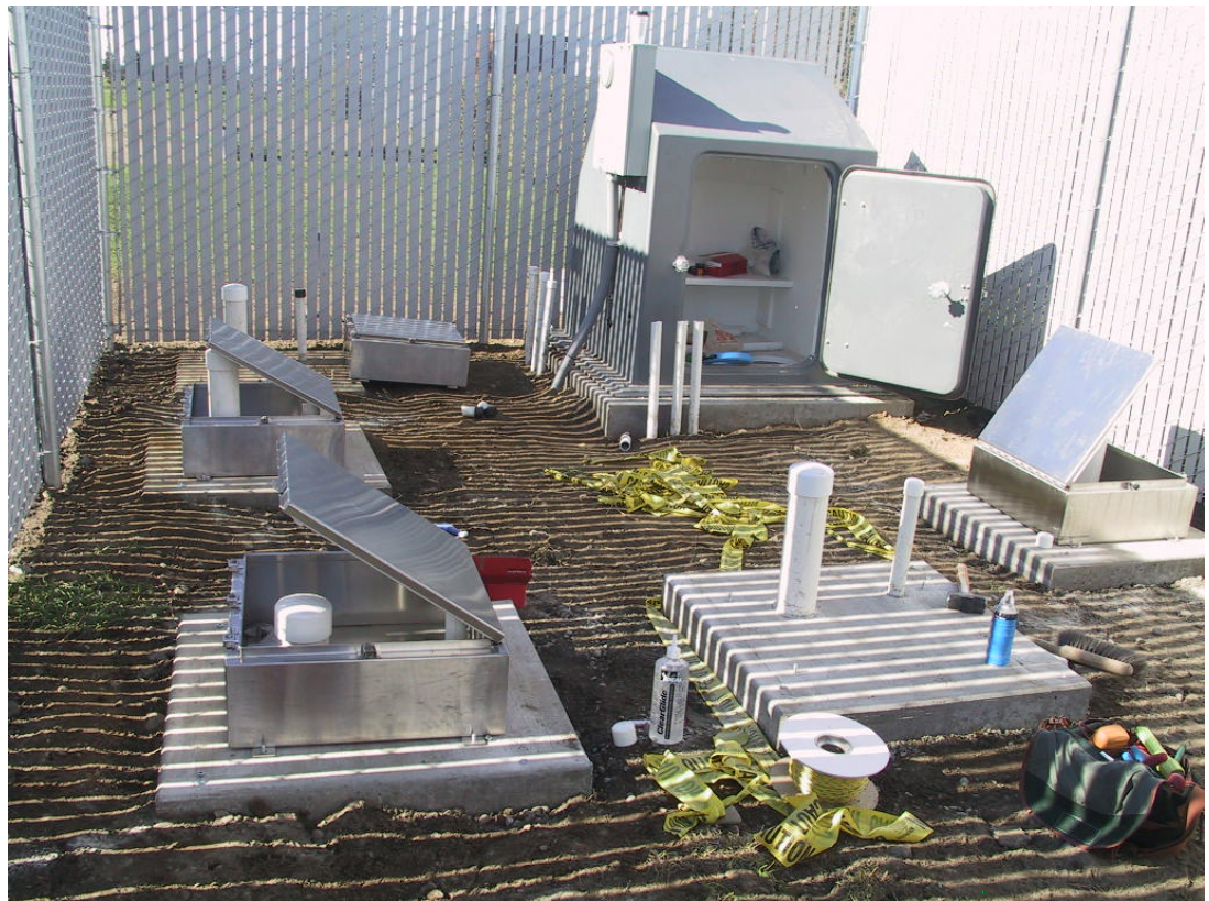
Figure 2. Delaney Park Geotechnical Array in Anchorage, Alaska. Photo shows locations of 5 boreholes and surface station (USGS photo)
