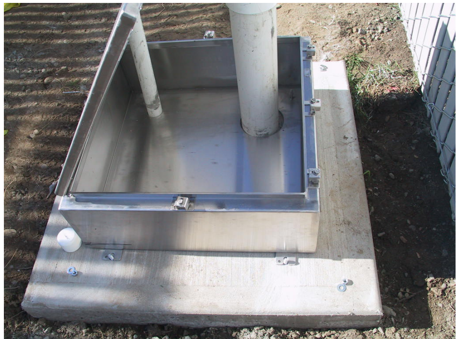
Figure 3. Stainless steel downhole sensor enclosure on the surface on concrete pad (USGS photo)
