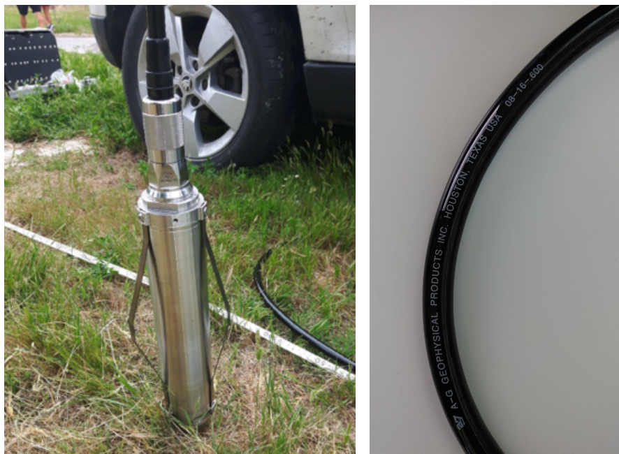
Figure 1. Sensor cable for borehole instrumentation (LUNITEK Photo)
